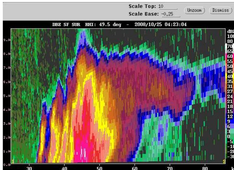
Fig. 41 : Vertical view of a supercell thanks to reflectivity
