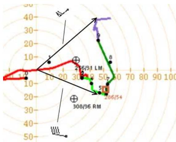
Fig. 18 : How measure speed and direction of wind with an hodograph
