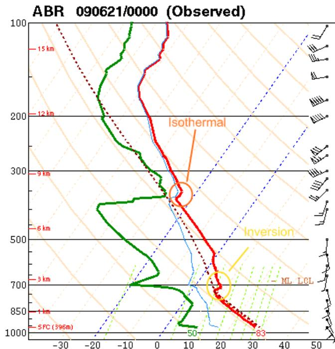
Fig. 27 : Example of sounding showing inversion and isothermal
