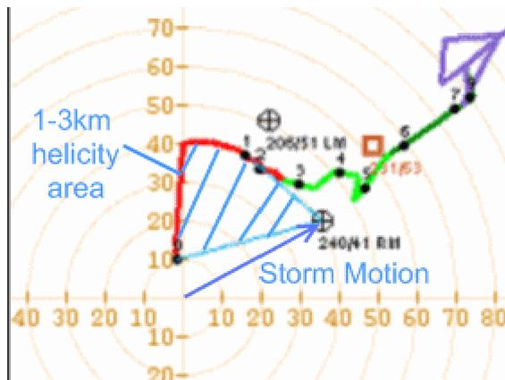
Fig. 28 : Picture representing an hodograph with storm motion and SRH
