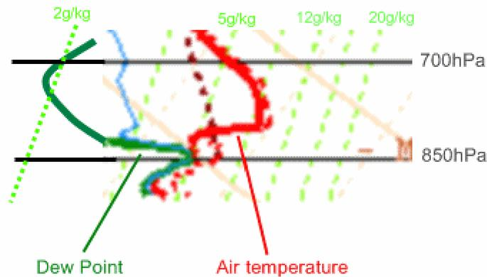
Fig. 23 : Picture showing the way to calculate RH
