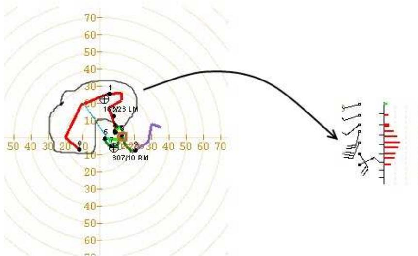
Fig. 17 : A color-coded example of a hodograph with corresponding winds (direction and speed)
