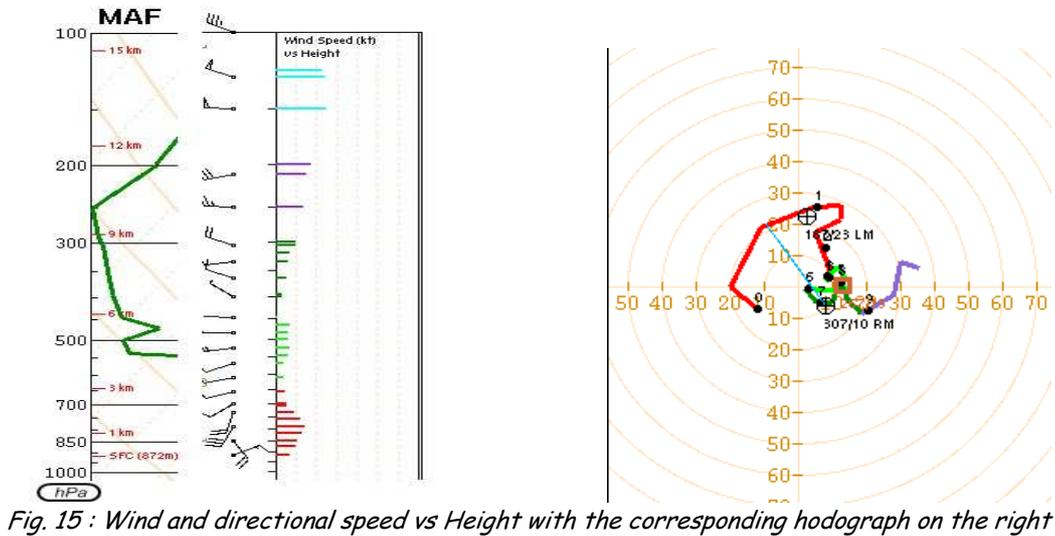
The picture on the left allows us to see the direction and speed of wind, according to altitude in hPa and correspondence in meters.
