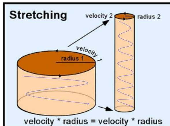
Fig. 48 : Stretching mechanism
