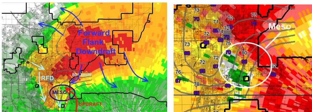
Fig. 42 : Diagrams showing different parts of structure supercell and the mesocyclone on the right picture
